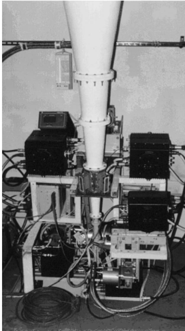
**Fig. 3.** S/X-band (3.5/13 cm) receivers of the Svetloe Observatory.
